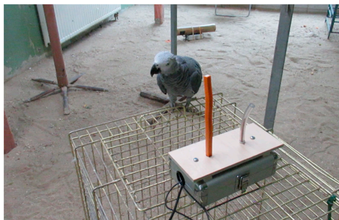
Figure 8. Prototype for a drum sequencer instrument with bending ruler.
