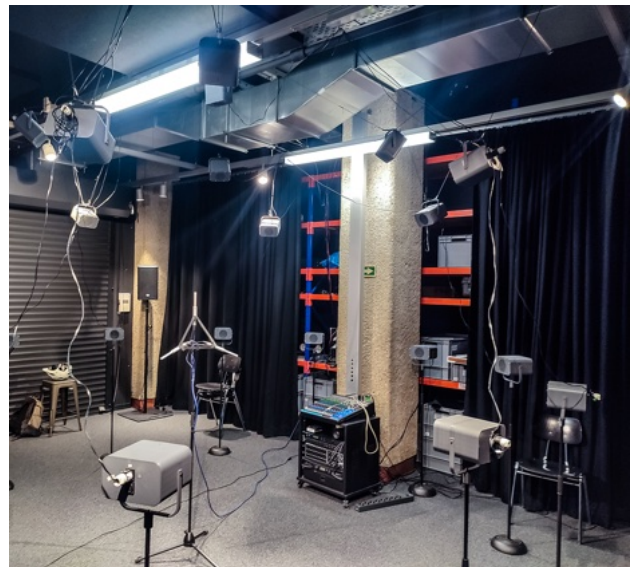
Figure 1. Test setup showing the tetrahedral microphone array positioned within a hemispheric 23-speaker array.
