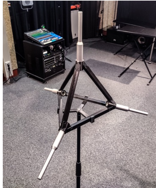
Figure 2. 3D-printed tetrahedral structure with outward-facing measurement microphones, designed to fit standard microphone stands.
