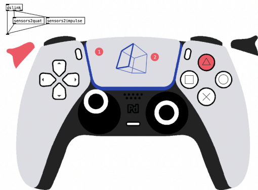
Figure 9: Screenshot of the [dsshow] object in Pure Data, displaying the controller state through input from a HID-based external.
